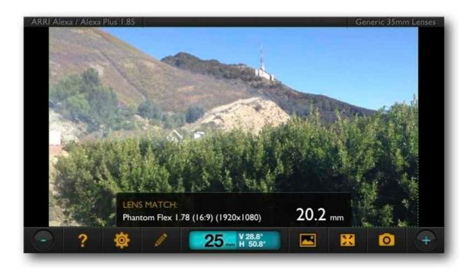
It's often the case that more than one format is being used on set. Using the Lens Matcher feature will calculate the equivalent focal length for your secondary format and display it for a moment on-screen as you change the focal length of your primary format.
