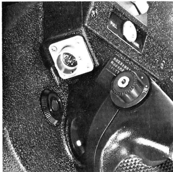
Fit the plug of the external battery box into the socket on the camera and turn it clockwise.
