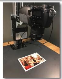
To adjust the camera height on the animation stand, squeeze the lock plate in, and gently slide the camera up or down.
