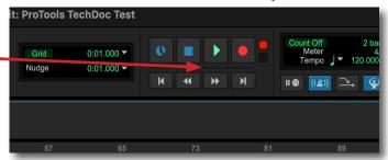
With your I/O selected and both record enable buttons active, you should now be able to monitor the sound coming into your microphone via the audio levels meter.
