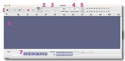
First, we will go to the Audio Setup pulldown menu (4) and select **Playback Device > Built-in Output**. This will direct audio to either your computers speakers or headphones, if a pair are connected to your computer.
