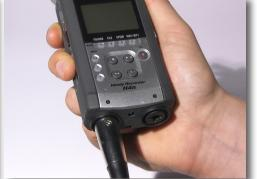
Gently press down on the "Power/Set" button on top of the receiver, and hold it down while the display reads WAIT.
