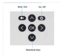
Observe the image being projected, and with the directional keys navigate to the "Digital Input" icon, and select it with the middle button
